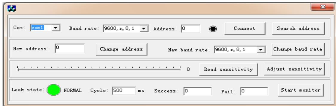
Choose the correct serial port number, baud rate and address click "Connect", make sure the computer and AG-LC1A Communication connection set successful.
